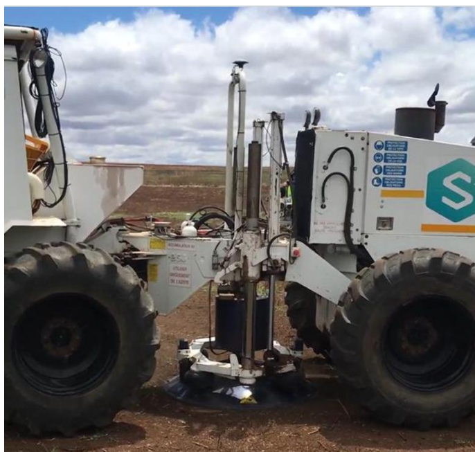
Figure 2 - Vibroseis vehicle on site, provide by EIMS.
